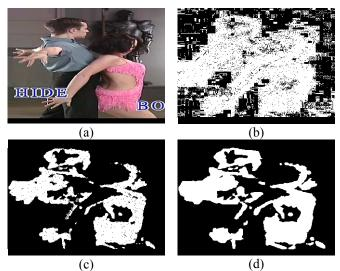
Fig. 16. (a) The original field, (b) The original-field difference, (c) The field difference after erosion, (d) Noise reduction after morphological reduction.
