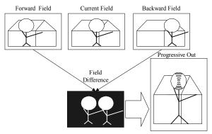
Fig. 10. The 2-field motion detection.
