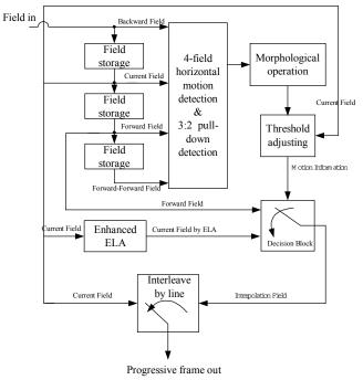
Fig. 5. Block diagram of proposed deinterlacing method.
