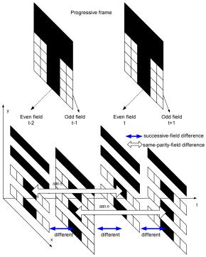
Fig. 9. 4-field motion detection in same parity.
