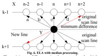
The minimum difference is chosen to be the highest correctional edge, and the opposite direction of the highest correction is used to detect a non-dominant directional edge region. As shown in Fig. 7, if the highest correction is a, then d and e are used for detecting the dominant edge region. The
