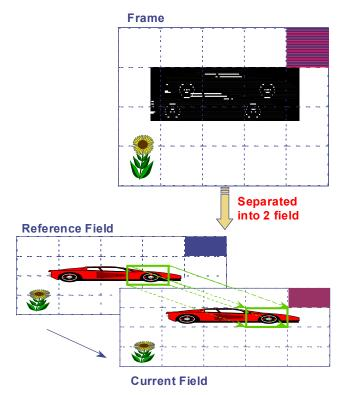
Fig. 4. Block matching by motion estimation method.
