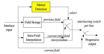
Fig. 3. Block diagram of motion adaptive deinterlacing.
